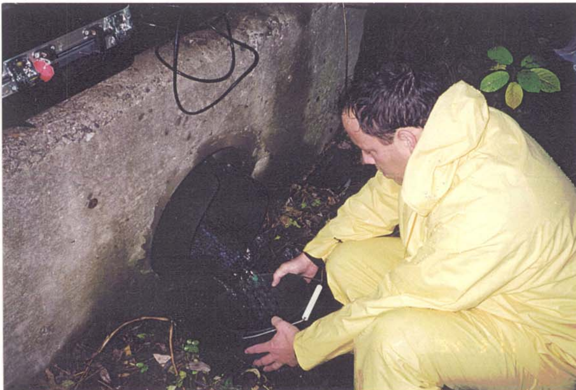
Figure 3-5: Flow measurements at the Cherry Hill site during low flow conditions. A flexible plastic sheet was placed into the existing pipe to create a lip. A graduated bucket was placed under the lip for flow measurements.
