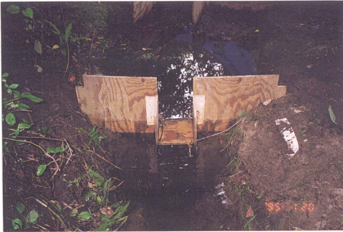
Figure 3-4: Flow structure at the Pinefield site for low flow conditions. The structure funneled the flow through a confined opening. The channel was excavated behind the opening to allow for the placement of a graduated bucket. Flow was measured by recording the time needed to fill the bucket.
