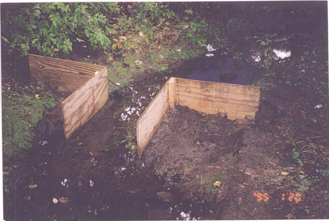
Figure 3-2: Flow structure at the Pinefield site for high flow conditions. The structure funneled the flow through a confined channel of uniform width. The natural base of the channel was flattened which included removal of rocks. The flow was measured by placing the Global Water flow probe into the middle of the channel.
