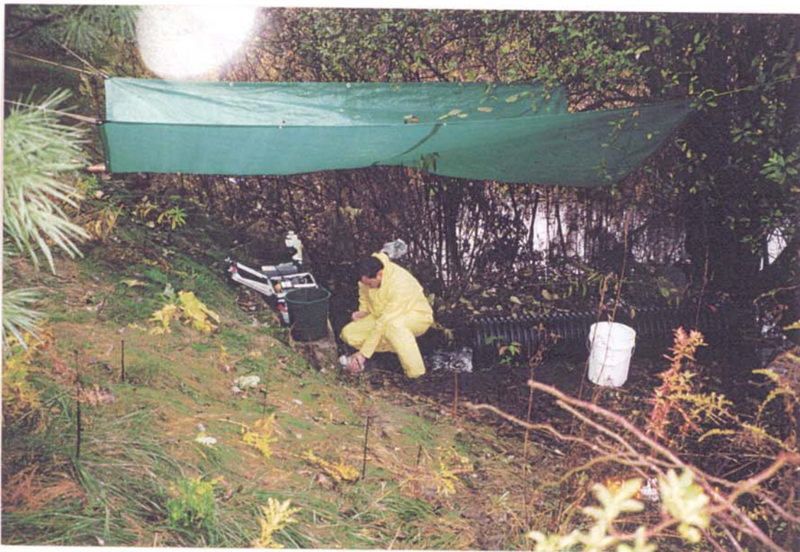
Figure 3-1: Stormwater sampling at the Cherry Hill site during Storm C. Water samples were collected by filling bottles without the use of a bailer.
