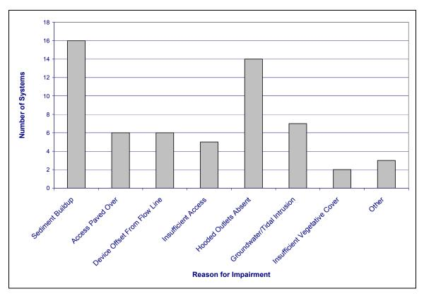
Figure 1. Causes of impairment to stormwater collection/treatment devices (note that some systems exhibit multiple causes of impairment)
