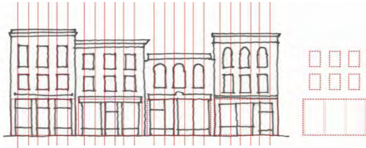
Rhythms and proportions of building modules, storefront modules and upper floor modules.
