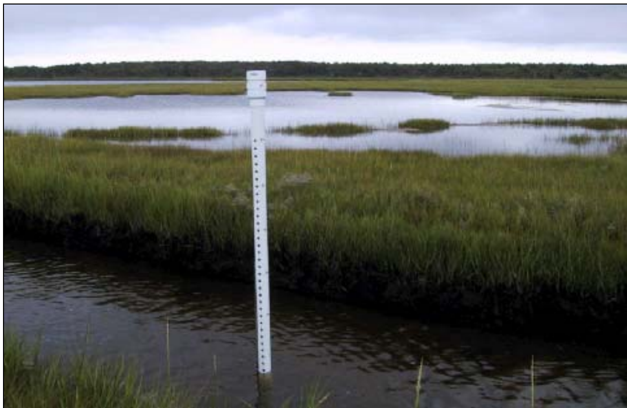
Figure 11. Tide height water level set-up for PTS and loggers.
