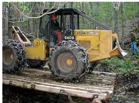
A temporary bridge allows machinery to cross water resources and minimize potential impacts.
