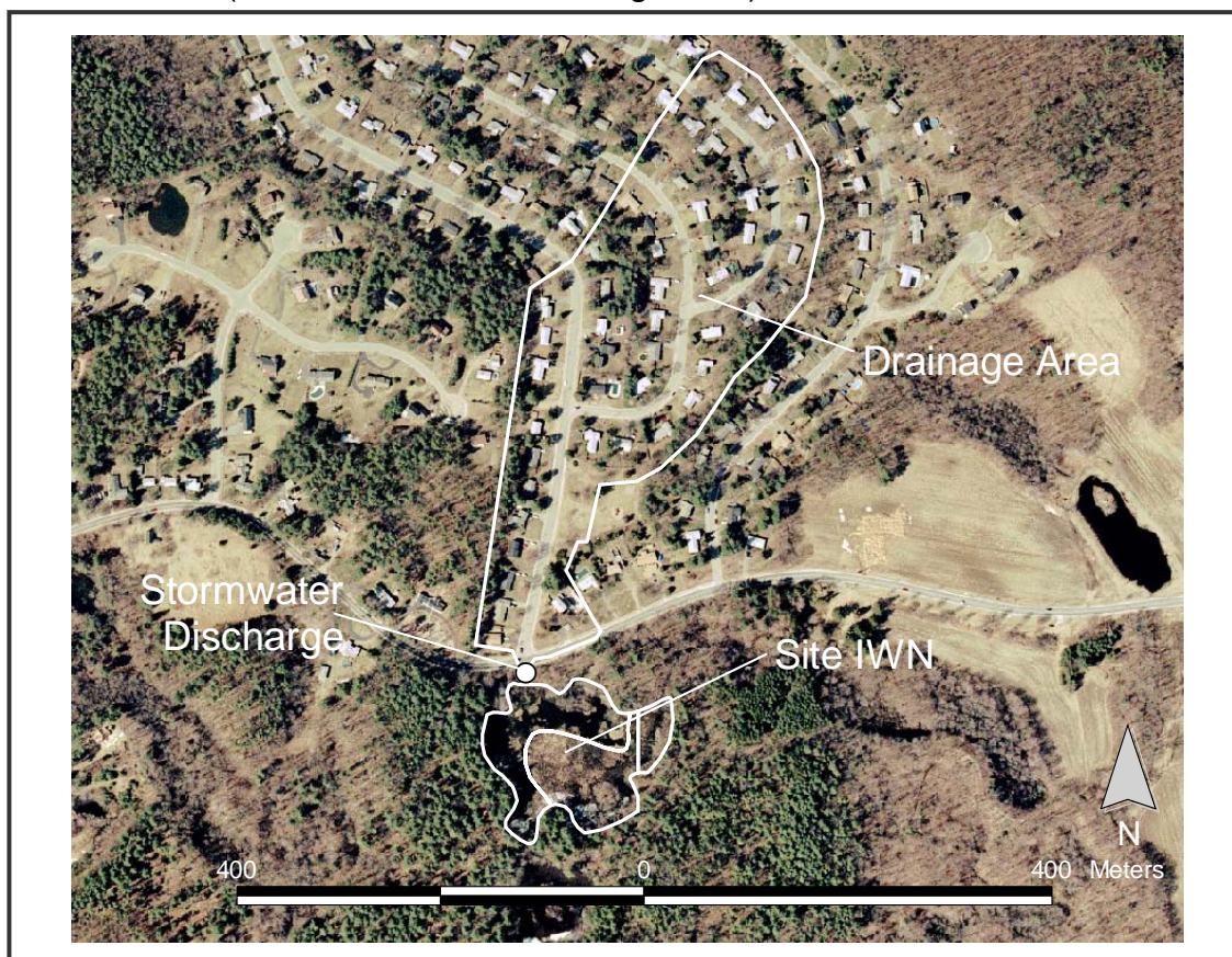
Figure 17. Site IWN, showing drainage area and discharge
