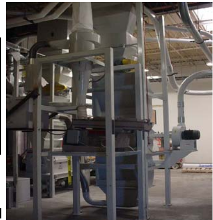
Right: Final step in grinding process at Sika Sarnafil
