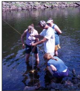
Martha Morgan, Doug Roberson, and Christina Bird learn to measure water velocity from USGS technician Linda Comeau during the RIFLS Certification field training.
