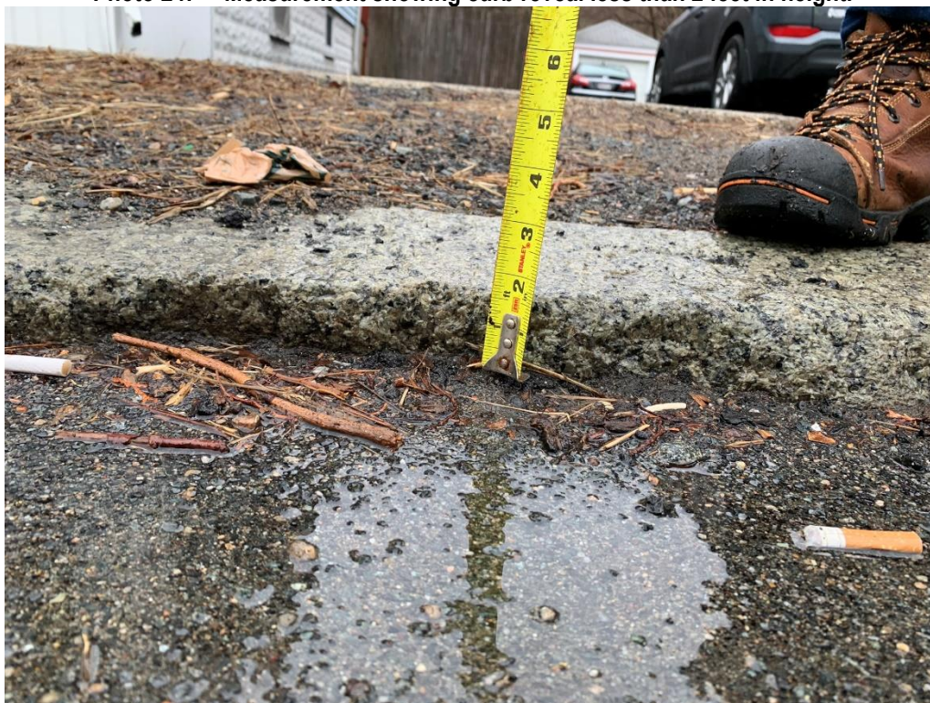
Photo 24: Measurement showing curb reveal less than 2 feet in height.
