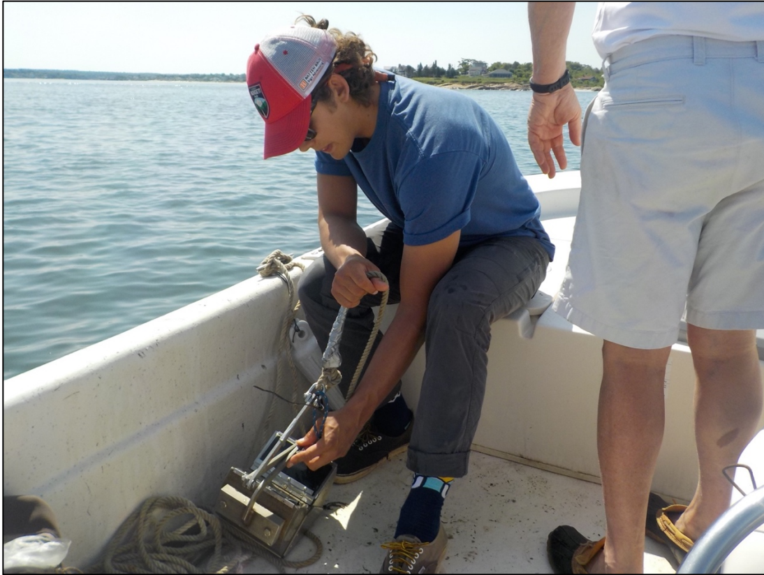
Figure 10. View of Ponar Grab sampler being armed
