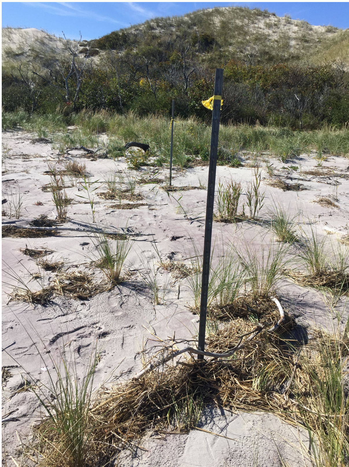
Figure 26. Close-up view of the metal fence post arrangement. This alignment aide the survey team run the same transit profile.
