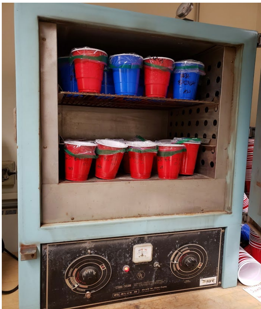
Figure 14. Photo of the oven used to dry the samples in the red cups.
