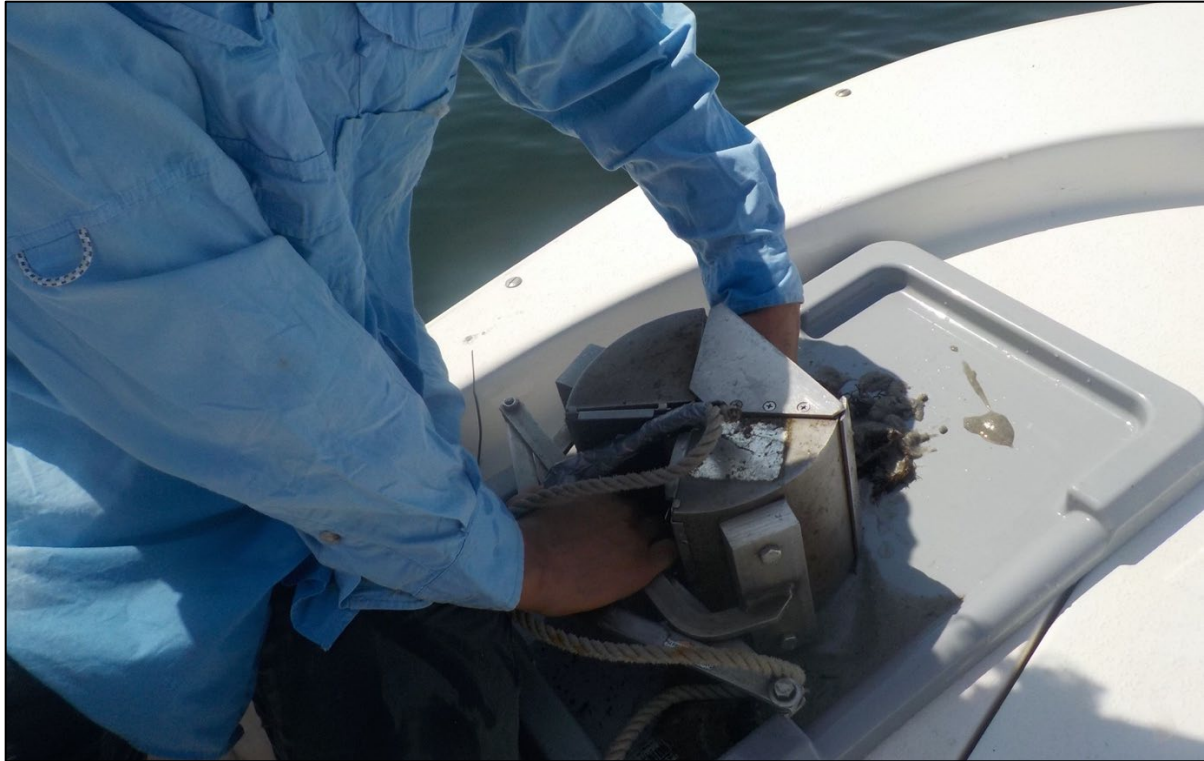
Figure 12. Grab is being to retrieve sand sampled.
