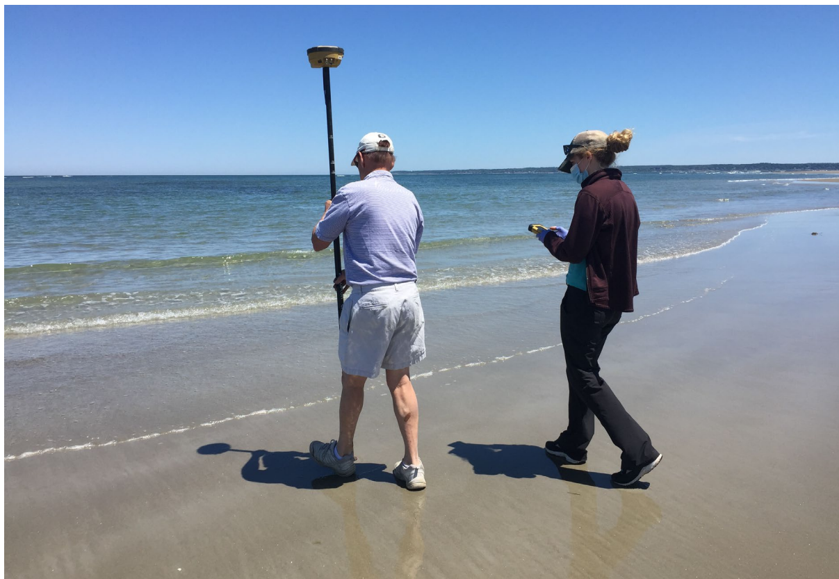
Figure 24. Scientists recording RTK beach profile survey.
