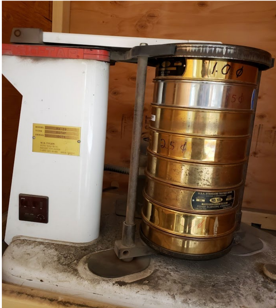
Figure 15. View of Ro-tap with nested brass sieves.
