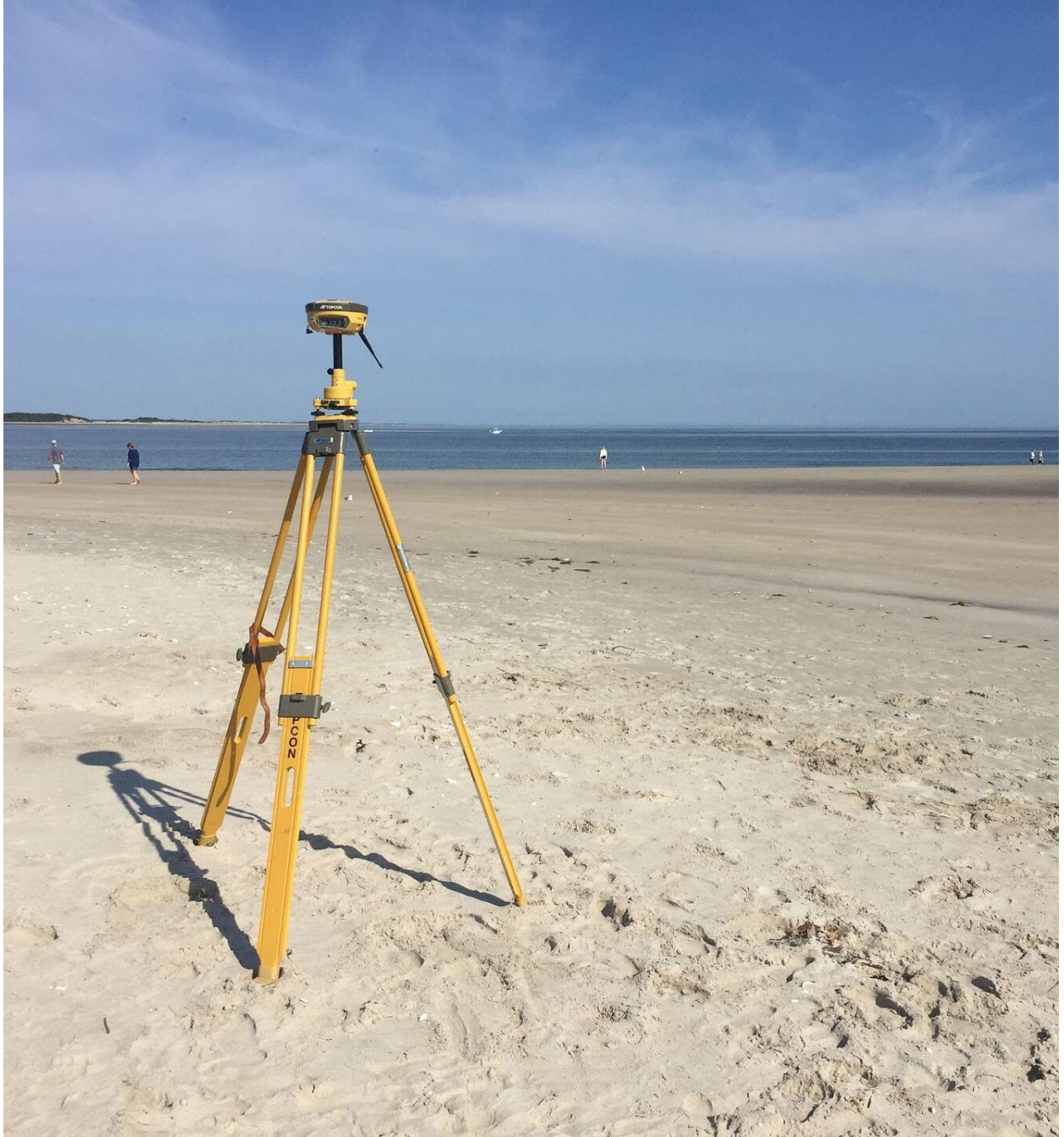
Figure 23. RTK Base station located at the mid-island beach protuberance. This site provided an unobstructed signal line to all the profiles.
