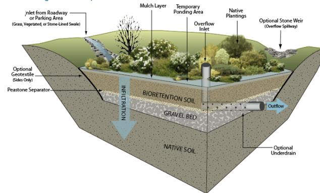
Image 2: Example of a parking lot with bioretention and diagram of a bioretention basin. Image source: MA Clean Water Toolkit.
