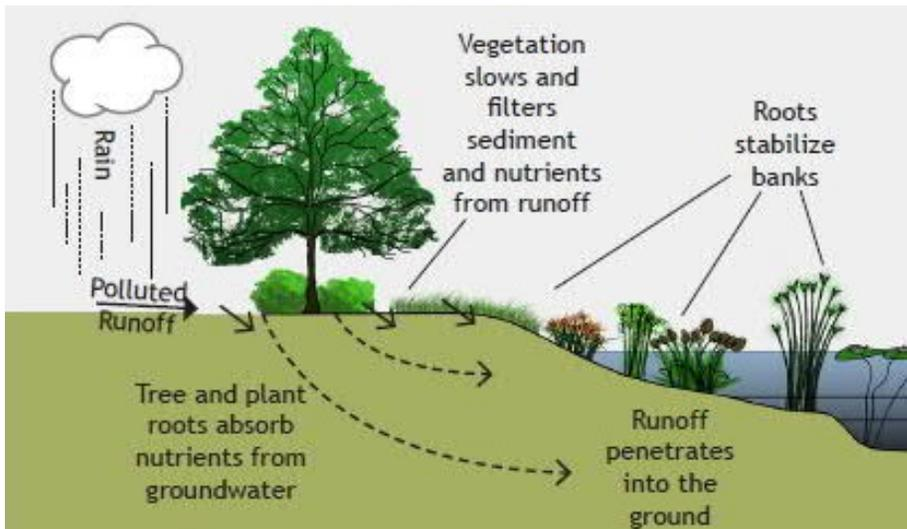
Image 1: Conceptual Diagram of a Riparian Buffer. Image source: <https://www.catawbariverkeeper.org/2017/04/25/nc-senate-passes-bill-eliminates-catawba-river-buffer-protection-prevents-local-water-quality-buffers/>
