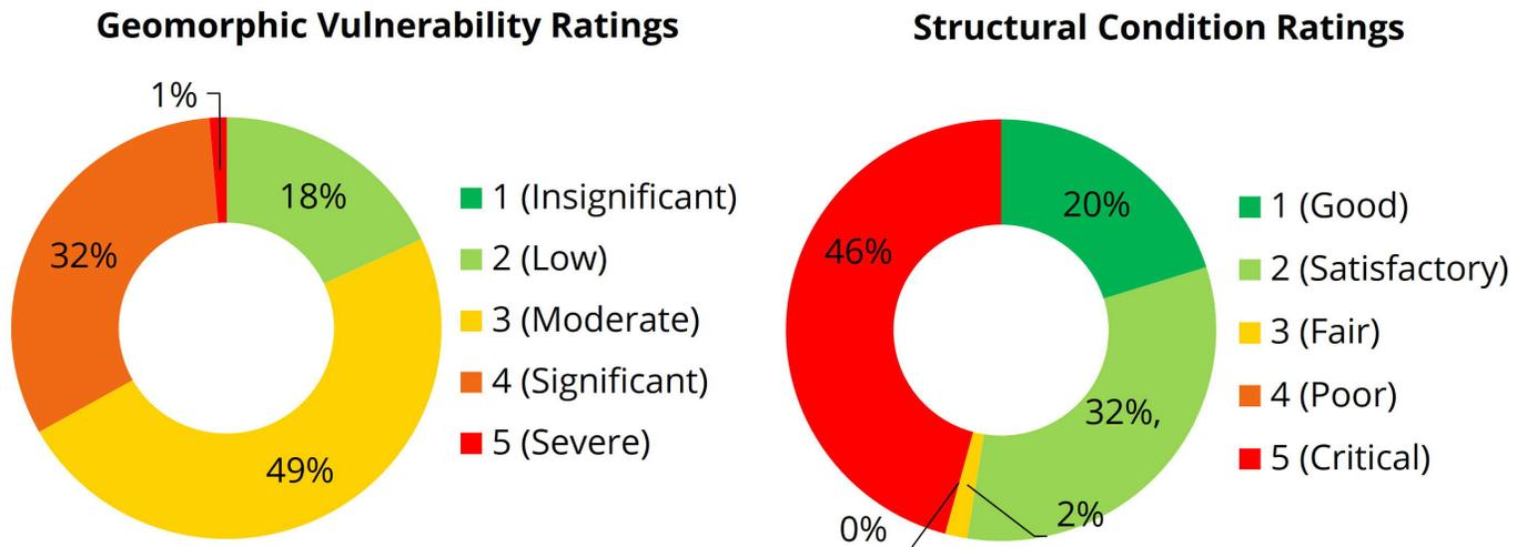
Figure 7. Distribution of geomorphic vulnerability and structural condition ratings across all assessed crossings.
