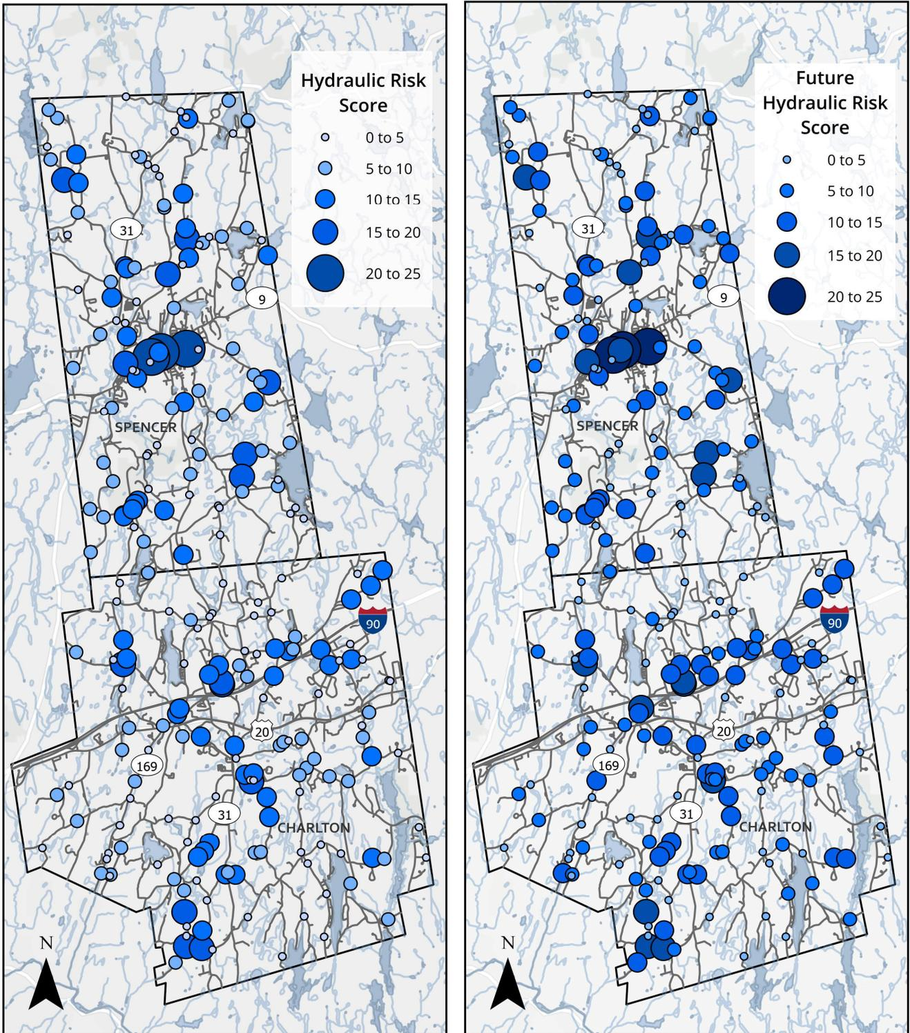
Figure 6. Spatial distribution of hydraulic risk scores for all assessed crossings under existing (left) and future (right) precipitation conditions.
