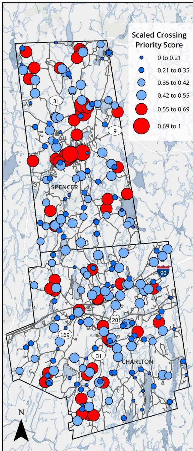
Figure 11. Spatial distribution of scaled crossing priority scores for all assessed crossings. Red dots indicate high priority crossings; light blue dots indicate medium priority crossings, and dark blue dots indicates low priority crossings.
