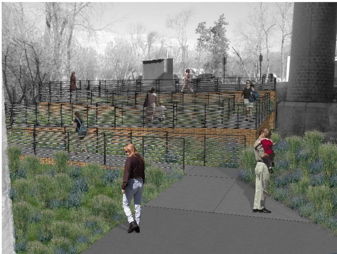
Image 2: Rendering of proposed ADA accessible pedestrian ramp with integral bioretention between the upper and lower parking lots.
