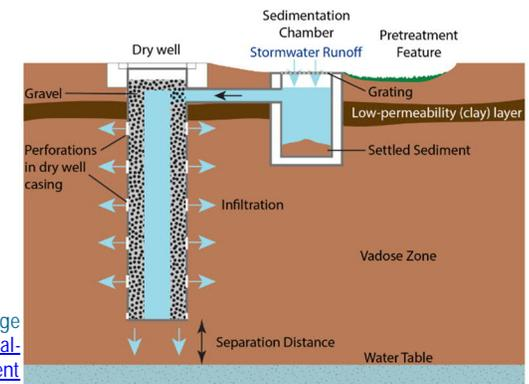
Image 2: Conceptual diagram of a dry well. Image source: <https://www.americangeosciences.org/critical-issues/factsheet/dry-wells-stormwater-management>
