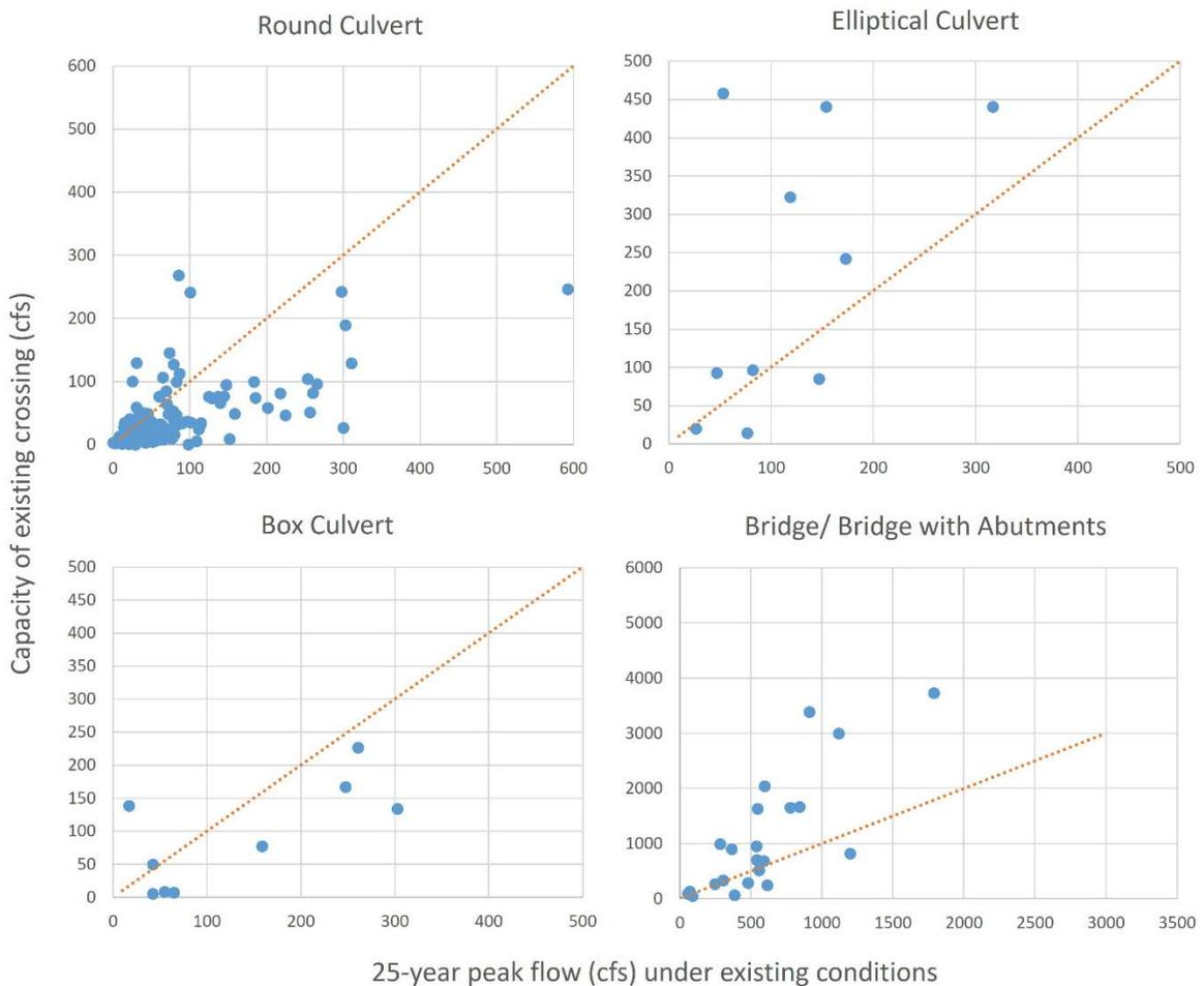
Figure 5. Capacity of existing crossings relative to the existing 25-year return interval flood, broken down by structure type. The dotted line in each panel represents the point at which capacity is matched to peak flows at a 1:1 ratio. Points above the line are sized with excess capacity for the 25-year return interval peak flow; points below the line have insufficient capacity to pass the 25-year return interval peak flow.
