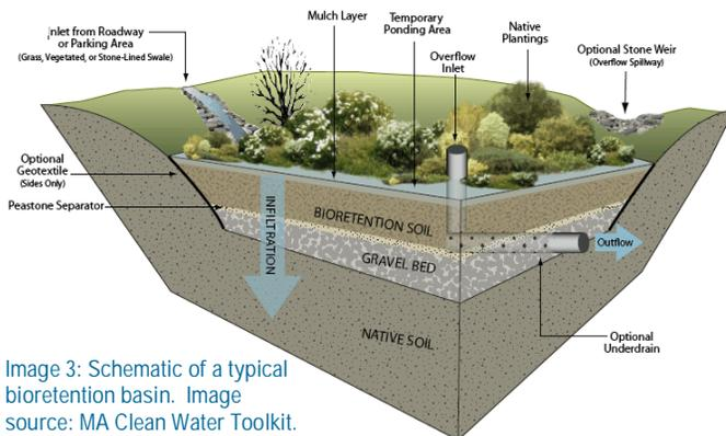
Image 3: Schematic of a typical bioretention basin. Image source: MA Clean Water Toolkit.
