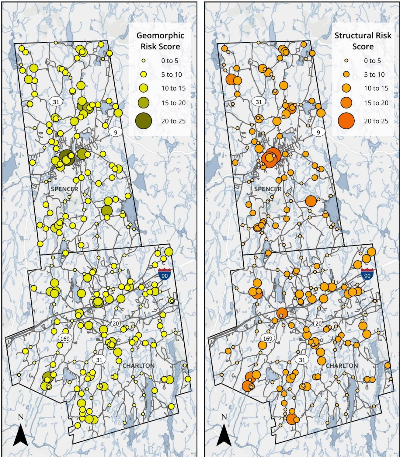
Figure 8. Spatial distribution of geomorphic risk scores (left) and structural condition scores (right) for all assessed crossings.
