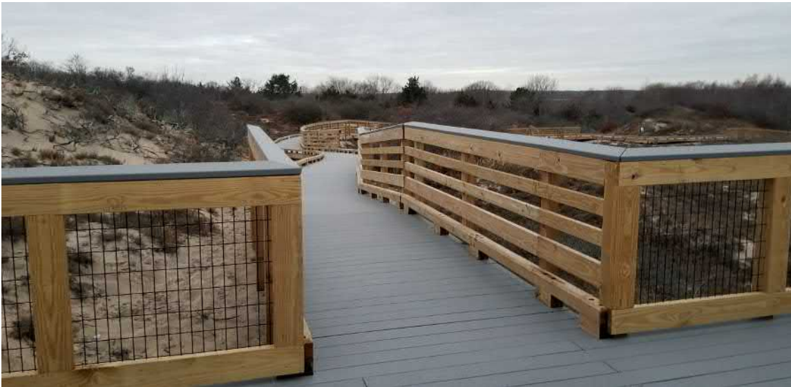
Figure 5. Example of an elevated walkway constructed of a combination of composite decking and wooden framing and handrails (Newburyport, MA).
