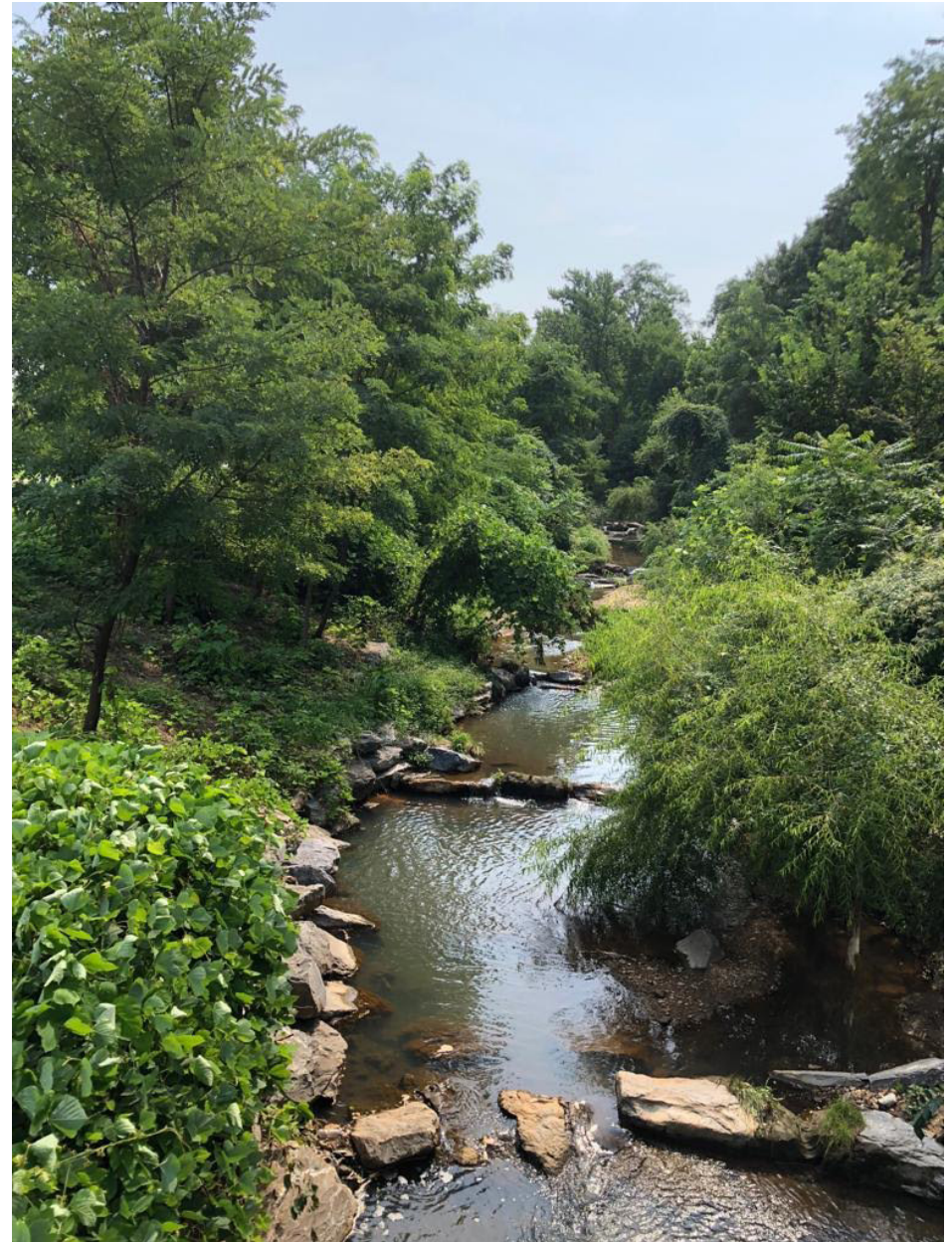
WATTS BRANCH STREAM RESTORATION PROJECT IN WASHINGTON, DC SHOWS CROSS VEINS DESIGNED TO SLOW STREAM VELOCITY AND BUILD UP VOLUME WITH THE INTENTION OF CREATING MORE DIVERSE HABITATS. PHOTO: J.FREY 2018
