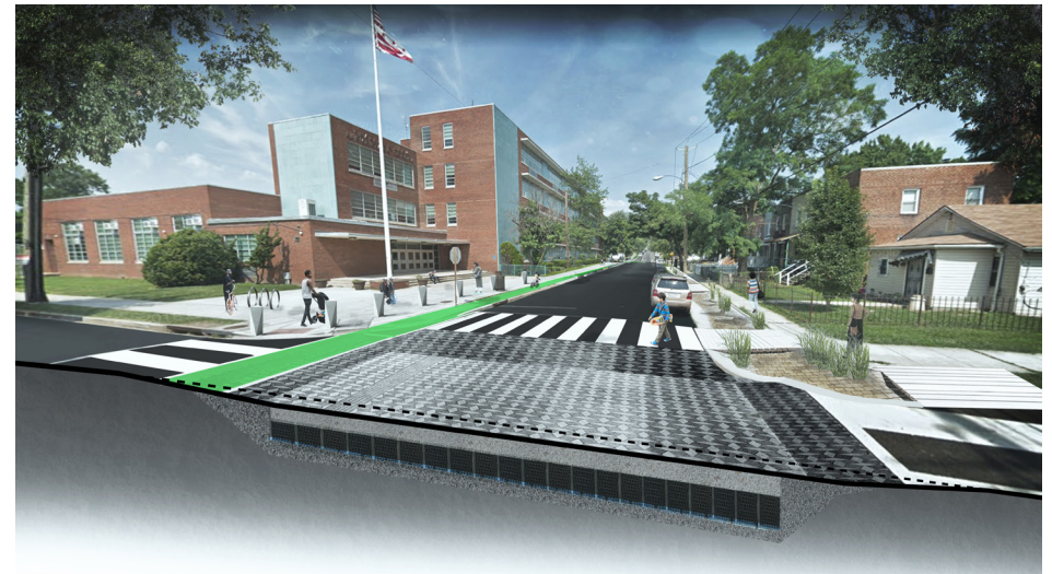
EXAMPLE OF PERMEABLE STREETS IN WASHINGTON, DC. INCLUDING STORMWATER CONVEYANCE, UNDERGROUND STORAGE, SLOWER ROADS NEARS SCHOOLS AND SAFER BIKING LANES.
