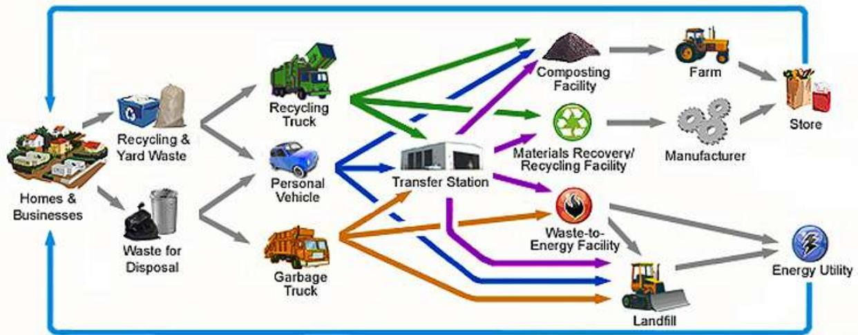
**Figure 4 Solid Waste Management System Material Flows**
