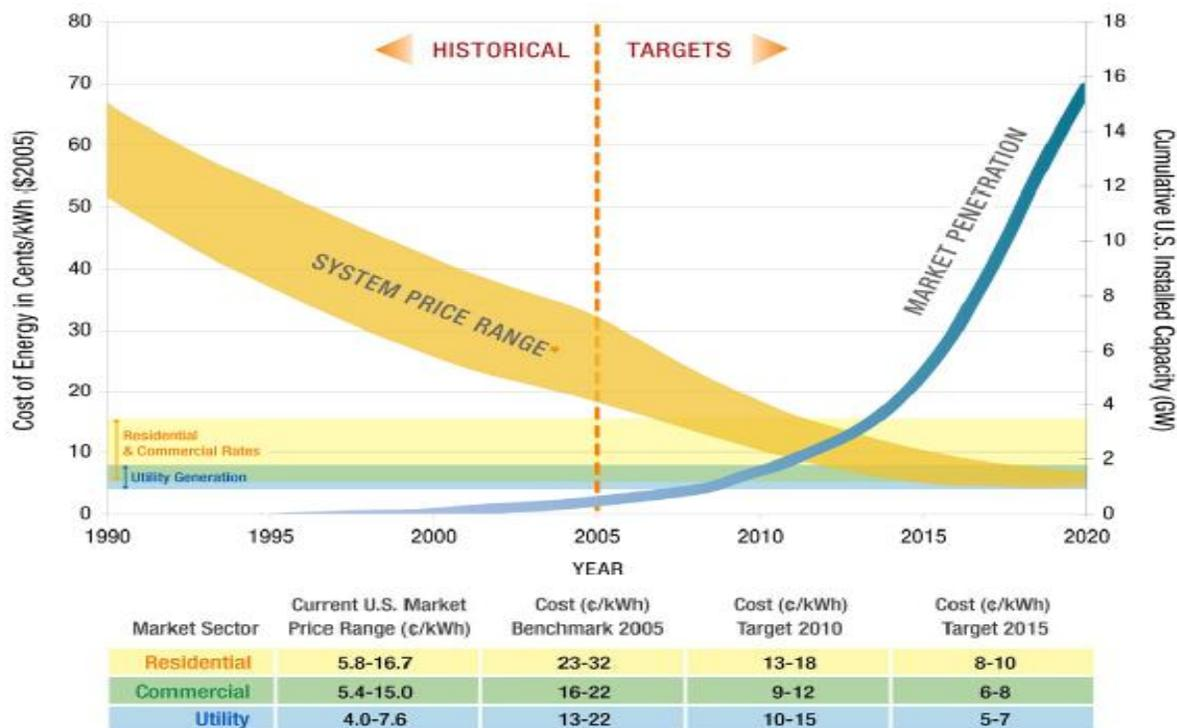
Figure 9 – Projected Future Costs of Installing Solar PV
