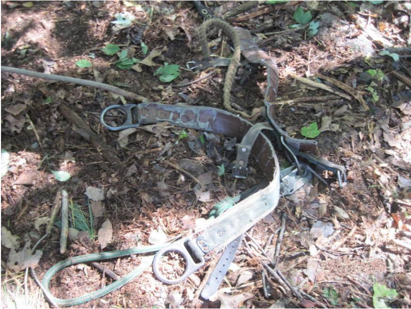
Figure 2 – Climbing gear that was in poor condition.
