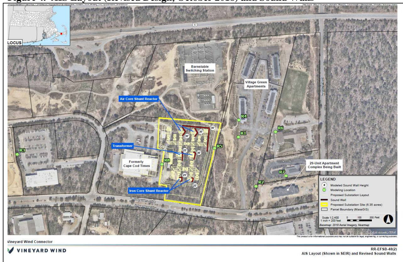
Figure 4. AIS Layout (Revised Design, October 2018) and Sound Walls
