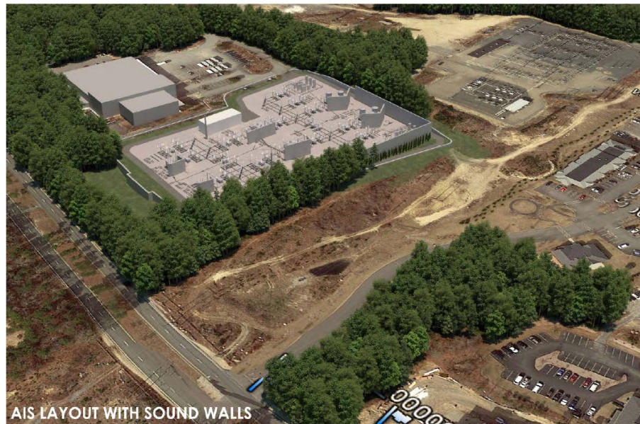
Figure 6. AIS Layout with Sound Walls
