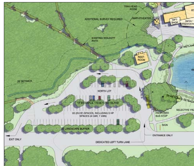
Proposed new layout for north parking lot showing pedestrian access to the new building (see Recommended Site Plan for relative scale, Pressley Associates)
