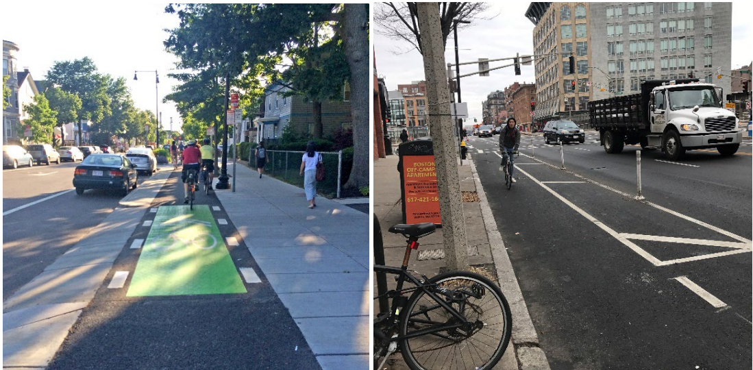
Protected/buffered bike lanes to reduce conflict points
