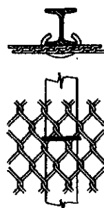
FASTENING FABRIC TO LINE POST, 5 mm STEEL CLIPS EVERY 300 mm±
