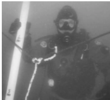
Left: DMF's Bob Glenn measuring the height of a lobster trawl groundline. Floating mainlines typically measured 5-6 ft. above the trap and increased to 16 ft. between traps.
