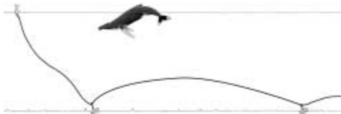
Diagram of lobster trawl rigged with "floating" groundline. Floating mainlines are now prohibited in Cape Cod Bay.
