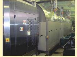
to gut and retrofit a 19th century building, and invest in a new Pulse-Flow continuous batch washing system that replaced eight regular industrial washer/extractors. ALADCO currently processes 600,000 pounds in linen products per month. The old process used 2.5 gallons of water per pound compared to 0.4 gallons today, 1,250,000 gallons of water saved each month. In addition to the reduction in water usage, there was a
