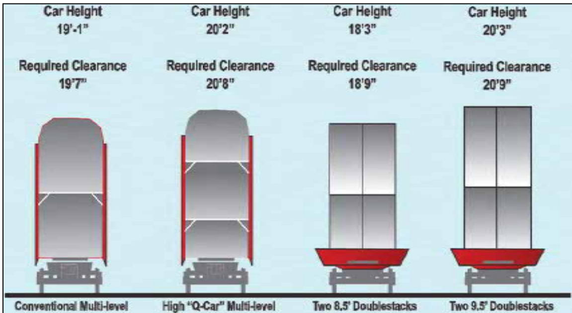
Figure 37: Auto Carrier and Intermodal Rail Car Clearance Requirements
