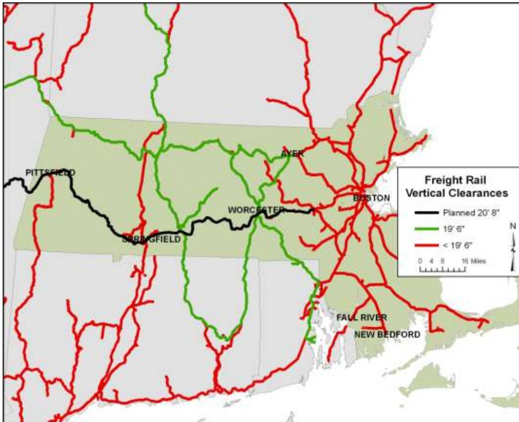
Figure 4-6: Auto Carrier and Intermodal Rail Car Clearance Requirements
