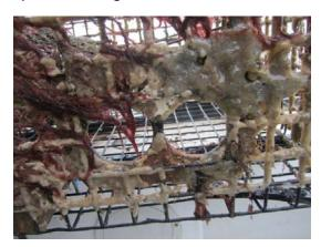
Figure 35. Escape vent/ghost panel of simulated ghost pot covered with tunicates and other organisms after nearly three years in the water.
