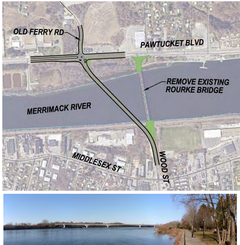
Figure 5-14 Alternative 6: Skewed Bypass Alignment
