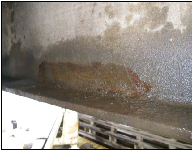
Figure 2-17 Typical Failure in Galvanized Coating
