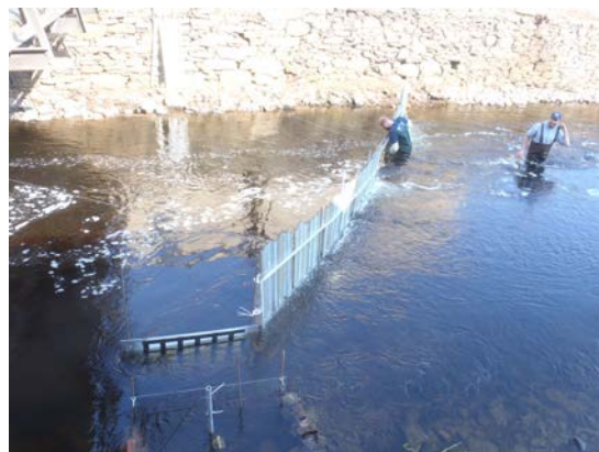
Figure 50. Biologists install a video counting system in the Mill River, Taunton.
