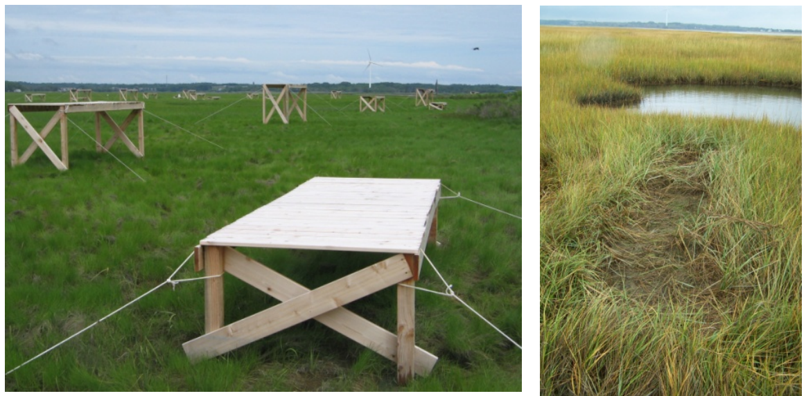
Figure 25. Dock shading study site in Marshfield (left) and the footprint of a 2 ft dock after end-of-season removal showing loss of vegetation due to dock shading (right).
