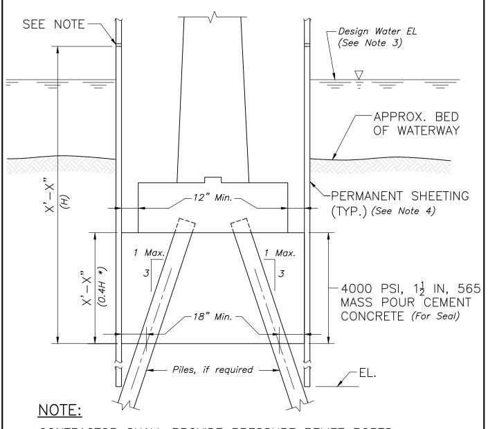
CONTRACTOR SHALL PROVIDE PRESSURE RELIEF PORTS LOCATED 2'-0" ABOVE DESIGN WATER LEVEL.
