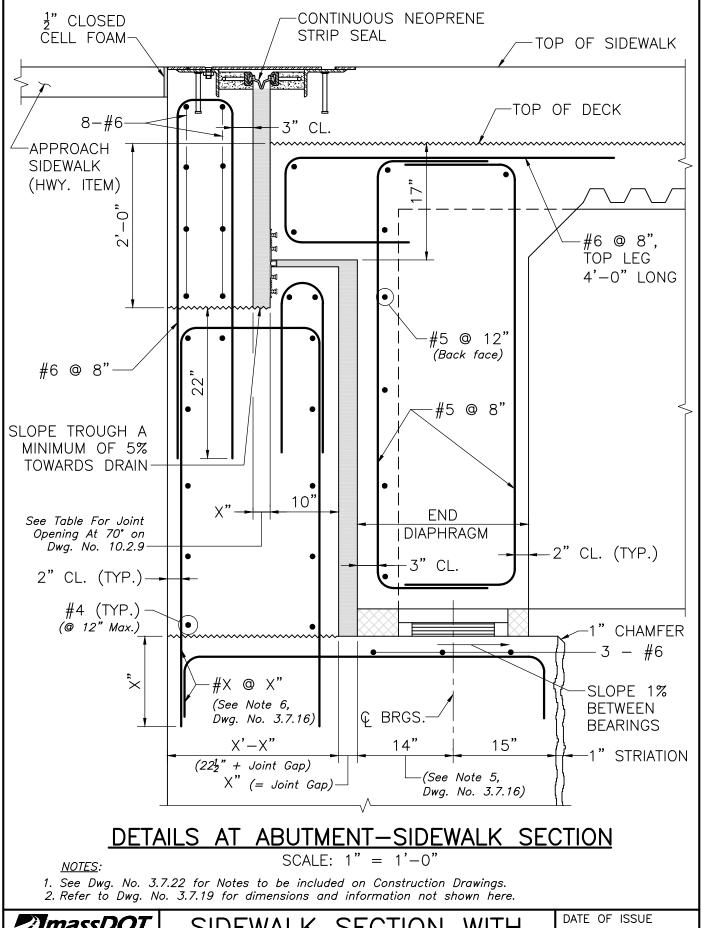
Imasspot LRFD BRIDGE MANUAL, PART II SIDEWALK SECTION WITH STRIP SEAL JOINT
