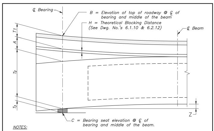
1. Bridge Seat Elevations shall be determined as follows:
