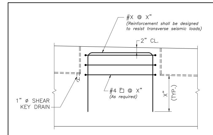
$\frac{\text{SECTION 4}}{\text{SCALE: 1"} = 1'-0"}$
