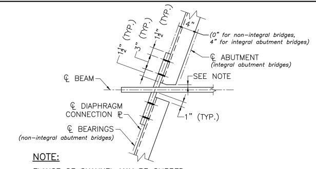
FLANGE OF CHANNEL MAY BE CLIPPED TO AVOID INTERFERENCE WITH WEB.
