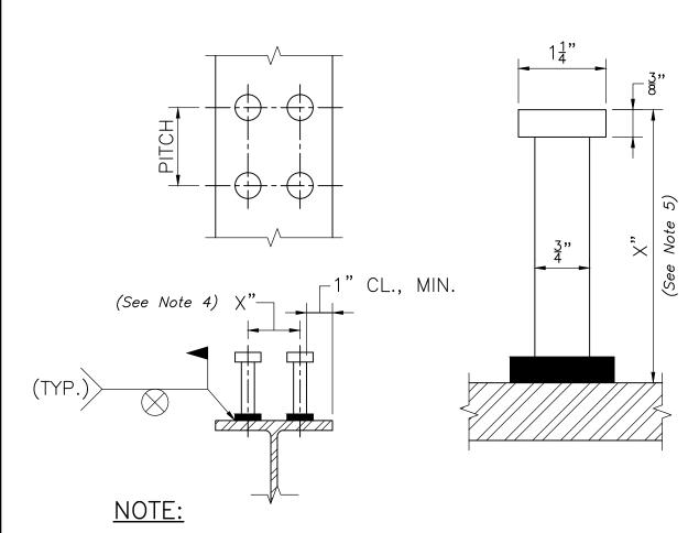
$\frac{7}{8}$ " ø studs may be substituted for  $\frac{3}{4}$ " ø studs by ADJUSTING THE PITCH TO PROVIDE AN EQUIVALENT CROSS-SECTIONAL AREA PER FOOT.
