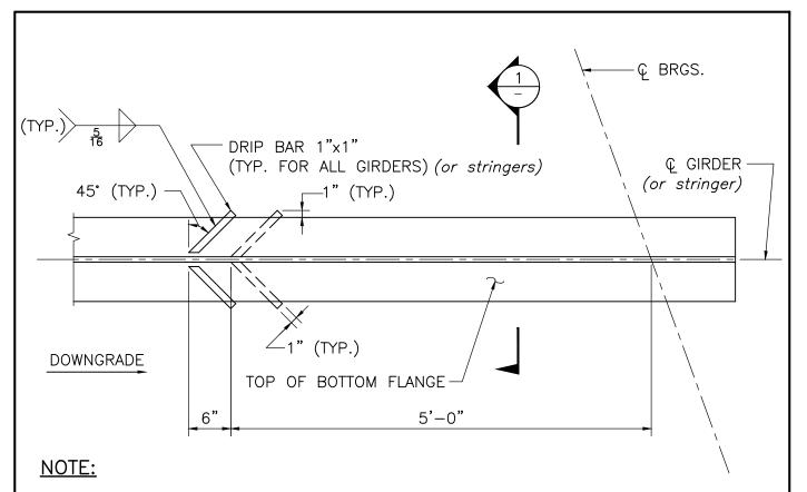
DRIP BARS SHALL BE LOCATED ON THE LOW END OF EACH SPAN FOR ALL GIRDERS (or stringers).
