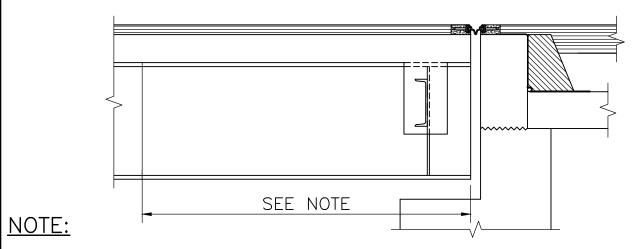
ALL UNPAINTED WEATHERING STEEL INCLUDING STEEL DIAPHRAGMS WITHIN 1.5 TIMES THE GIRDER DEPTH (7'-0" MIN.) OF BRIDGE EXPANSION JOINTS SHALL BE PAINTED IN ACCORDANCE WITH THE STANDARD SPECIFICATIONS. THE FINISH COAT COLOR SHALL MATCH COLOR CHIP NO. 30045 OF FEDERAL STANDARD 595B.
