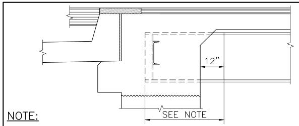
THE UNPAINTED WEATHERING STEEL STRINGER (or girder) AND ATTACHED PLATES EMBEDDED IN THE ABUTMENT (or in the concrete end diaphragm) AND WITHIN 12" OF THE ABUTMENT FACE (or face of the concrete end diaphragm) SHALL BE PAINTED IN ACCORDANCE WITH THE STANDARD SPECIFICATIONS. THE FINISH COAT COLOR SHALL MATCH COLOR CHIP NO. 30045 OF FEDERAL STANDARD 595B. THE STEEL DIAPHRAGM SHALL NOT BE PAINTED.
