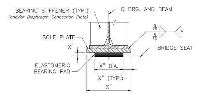
(\*) – WELDS SHALL TERMINATE  $\frac{1}{4}$ " FROM EDGE OF PLATE.
