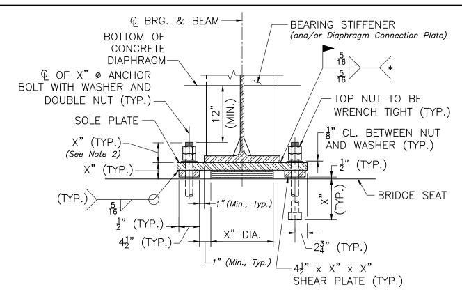
(\*) — WELDS SHALL TERMINATE ¼" FROM EDGE OF PLATE, MASKING AND TOUCH—UP PER STANDARD SPECIFICATIONS.
