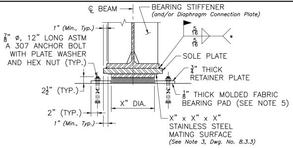
(\*) — WELDS SHALL TERMINATE  $\frac{1}{4}$ " FROM EDGE OF PLATE, MASKING AND TOUCH—UP PER STANDARD SPECIFICATIONS.
