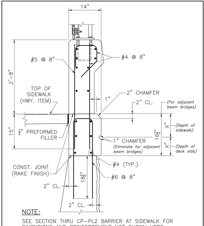
DIMENSIONS AND REINFORCEMENT NOT SHOWN HERE.
