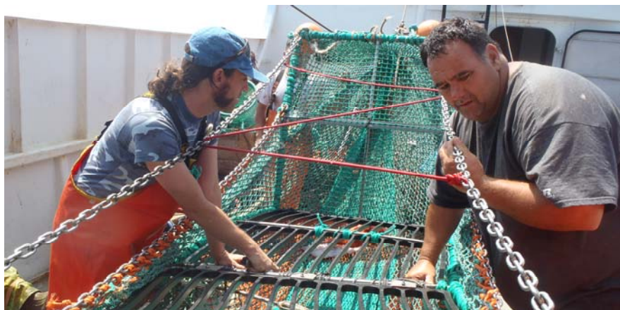
Figure 10. David Chosid and Mike Walsh make adjustments to a sorting grid system designed to reduce catches of small redfish.
