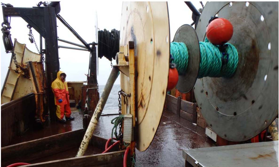
Figure 8. CE collaborated with SMAST to test a semi-pelagic trawl with low seabed impact to target haddock and avoid overfished flounders. The image shows the compared gear types: standard bottom contact trawl doors (inside the vessel) and standard ground gear (aft drum) vs. semi-pelagic doors (outside the vessel) and floating bridles (forward drum).
