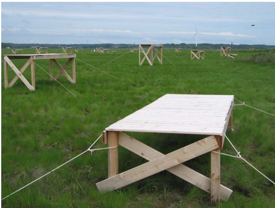
Figure 21. A view from the high marsh of the experimental dock shading study site in Marshfield. Docks were installed over the marsh during the growing season from 2013–2015. Four foot wide docks were set two, four, and six feet above the marsh platform to assess the relative shading impacts of docks relative to the 1:1 height to width ratio guideline for dock construction over salt marsh.
