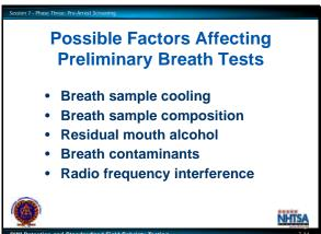
Radio frequency interference (RFI) can produce either high or low test results, or can prevent a breath test device from producing any result. Care should be exercised when utilizing a PBT around radio equipment.
