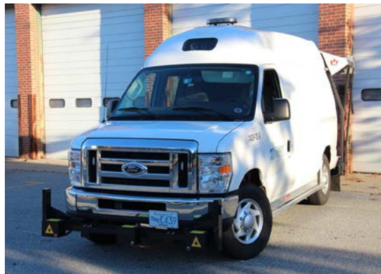
Figure 5- Pavement Management Vehicle
