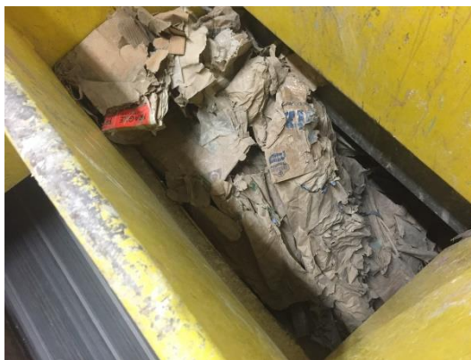
Figure 2 – OCC Chute off Mixed C&D Processing Line
