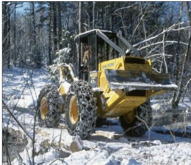
Skidder on a temporary bridge
