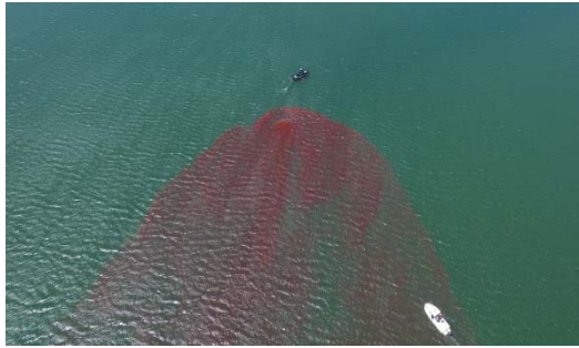
Figure 9. Image of effluent and Rhodamine dye boiling to the surface from the end of the Plymouth Waste Water Treatment Plant outfall pipe in Plymouth Harbor. Photo courtesy of Brewster EMS.
