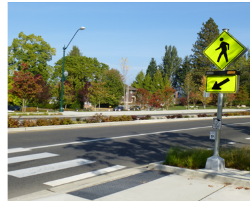
Figure 7. Example of a hybrid beacon (top) and an RRFB (bottom)
