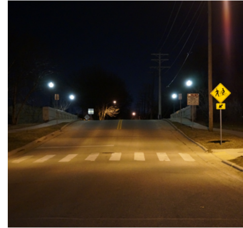
An example of a well-lit crosswalk and a sidewalk with pedestrian scale lighting.
