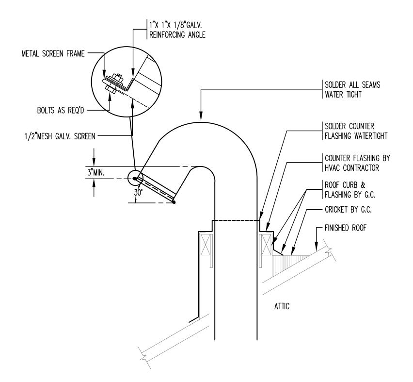
TYPICAL ROOF GOOSENECK DETAIL
