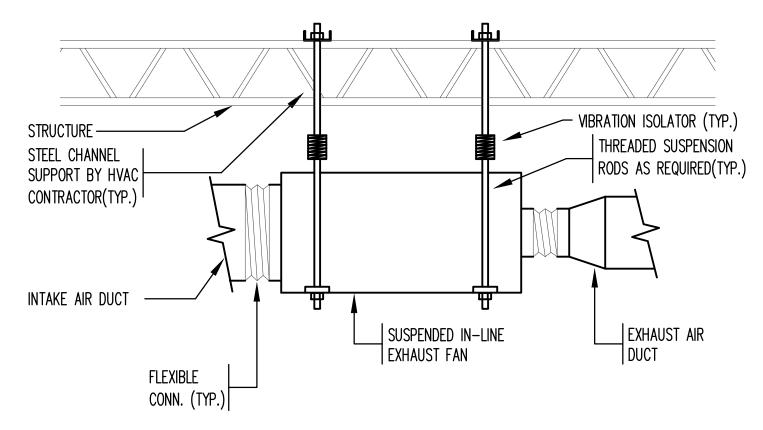
SUSPENDED IN-LINE EXHAUST FAN DETAIL
