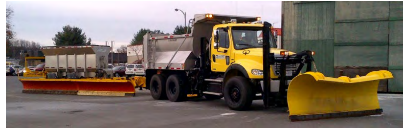
MassDOT 10-wheel dump truck equipped for snow & ice with tow plow
