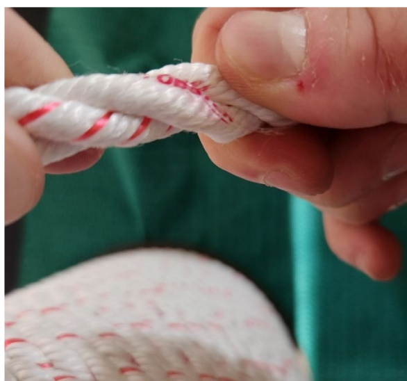
Figure 39. Everson whale-safe weak rope with “MASS LOBSTER” ribbon.
